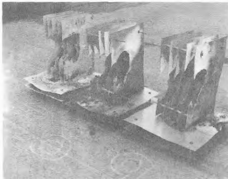
Fig. 12 - Extinguished standard magnesium sheets
